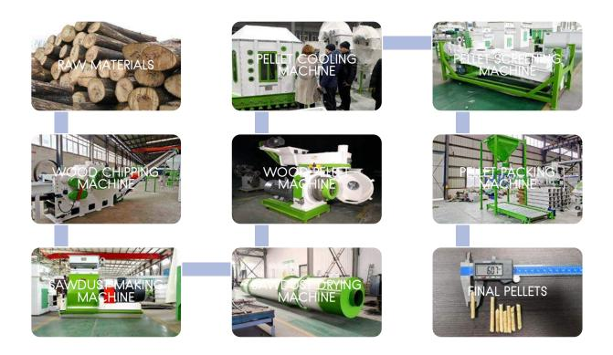
Raw materials such as wood or other forest wastes cannot be directly pelletized if they are large in size. They need to be sliced and crushed to be processed into 3–5mm sawdust.
